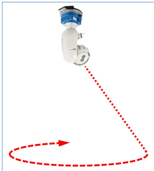
Figure 58 Horizontal scan coverage
